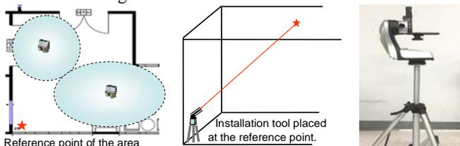
Fig. 3 Laser pointer: a BeDIPS installation tool
