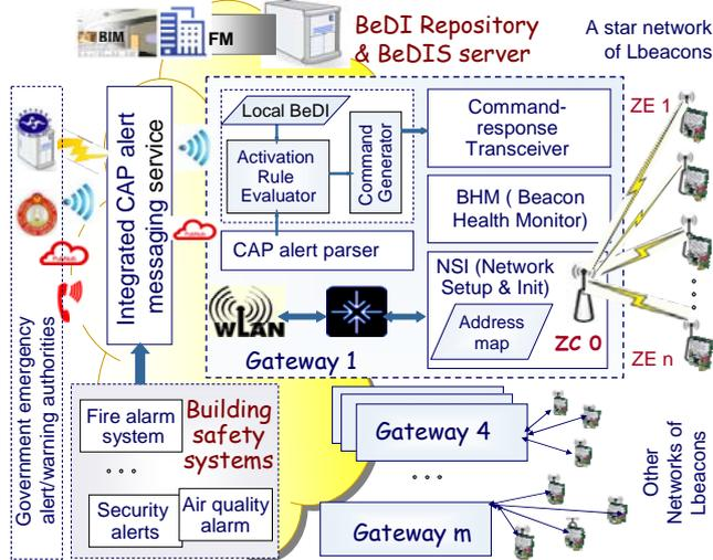
Fig. 8 Structure of BeDIS
