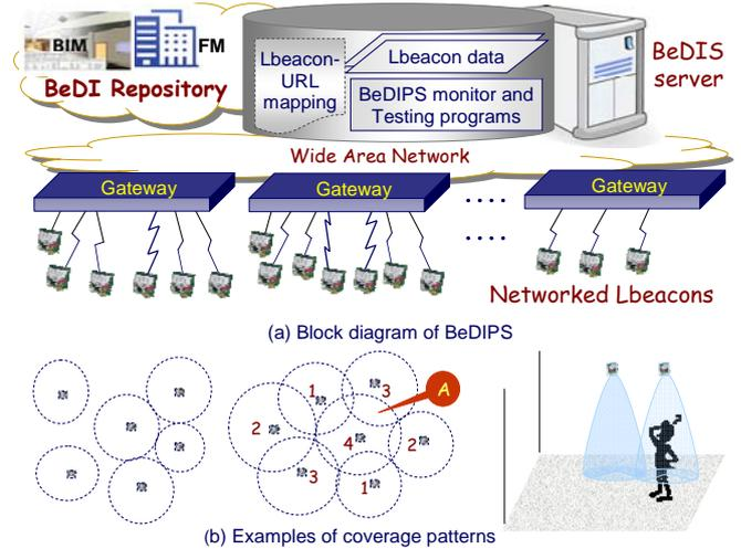
Fig. 4 Structure of BeDIPS and Lbeacon coverage
