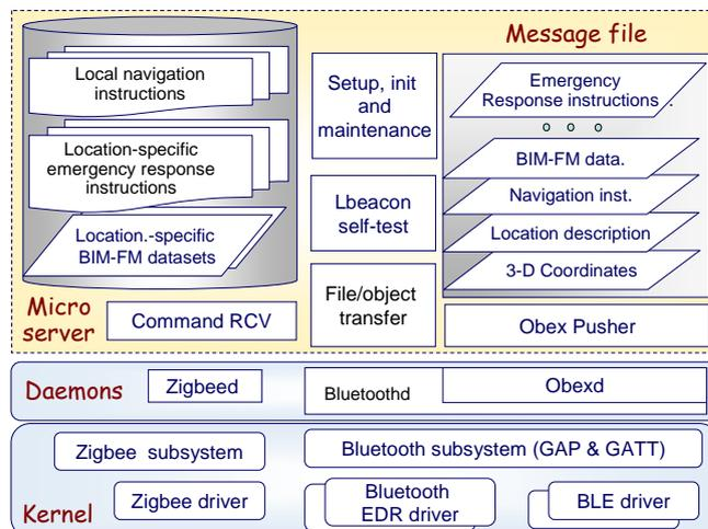
Fig. 10 Structure of Micro BeDI server
