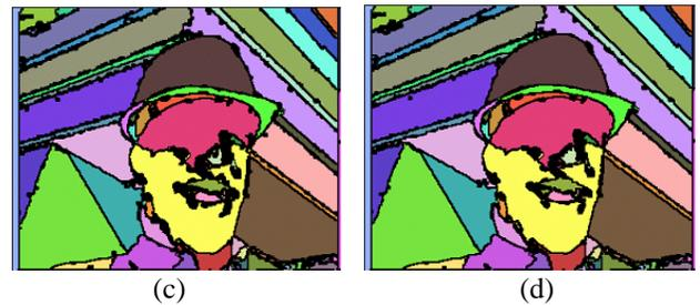
Fig. 4. Markers extracted from frame 116 of sequence “foreman” with different the value of  $k$  after Step 1.2 for marker extraction. (a)  $k = 0.8$ . (b)  $k = 1.0$ . (b)  $k = 1.2$ . (b)  $k = 1.4$ .
