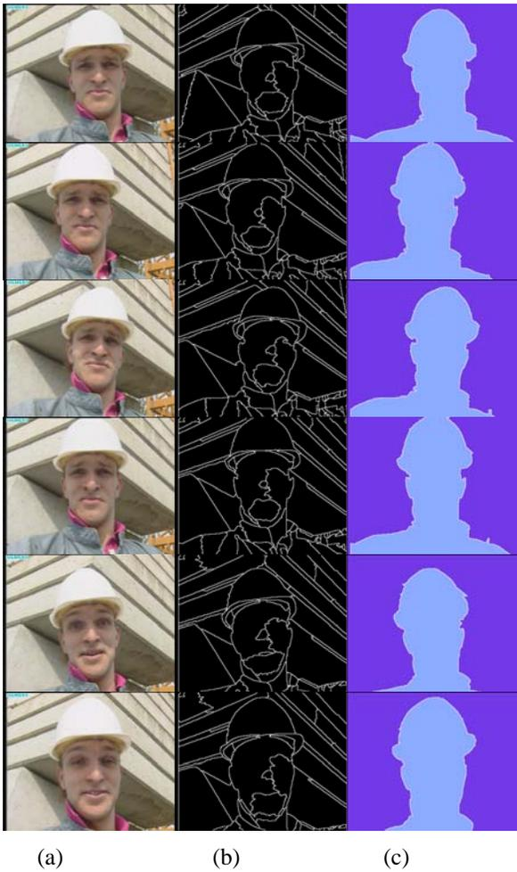
Fig. 9. "Foreman" sequence: Frame 1, 20, 40, 60, 80, 100. (a) Original images. (b) After temporal tracking. (c) After Bayesian merging.
